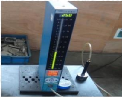
Use air gauge to do 100% inspection hole diameter after finished boring 用气孔量仪对孔径做100%检查
