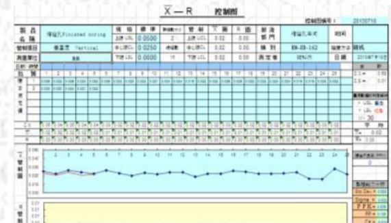
Key dimension by X-bar chart control 关键尺寸用X Bar控制图
